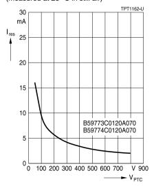
Minimum resistance of PTC thermistors versus applied voltage (pulsed)
