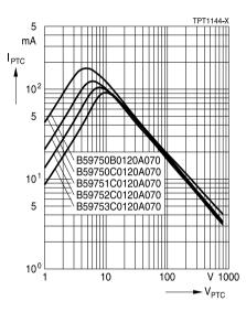
Residual current in high-ohmic state  $I_{res}$  as function of applied voltage  $V_{PTC}$ , typical (measured at 25 °C in still air)
